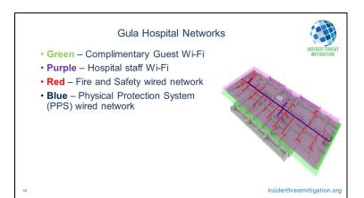
**Red** – Fire and Safety wired network. Enables fire sensors and life monitoring devices to communicate with nurse station.
