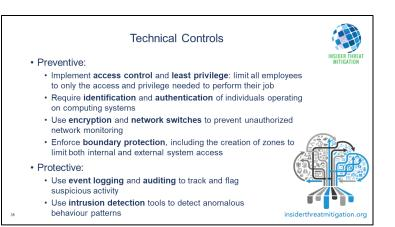
snooping. We should also install firewalls and data diodes to enforce network separation and boundary protection. Finally, we need to collect computer events and auditing to flag suspicious activity. We should also implement intrusion detection tools to look for anomalous behaviour. Of course, if we don't regularly look at these events, audits, and intrusions, they aren't effective.
